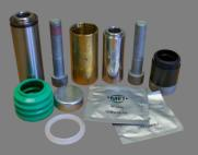
**5R0200** Guide Pin Kit for LB195 and LB225 MEI Calipers. Suitable for KB Calipers kit number K001915
