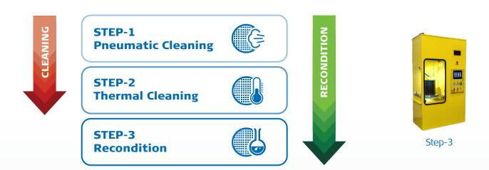
Normal cleaning includes only step-1 and step-2 using pneumatic and thermal cleaning to remove loose ash and to partly remove hardened ash.
